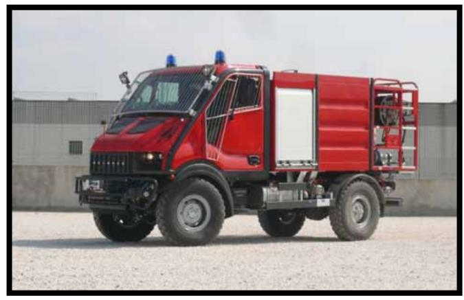
Steel (or Alluminum) Water tank capacity **2.000 liters**Centrifugal water pump driven by T-REX T-BOX PTO
