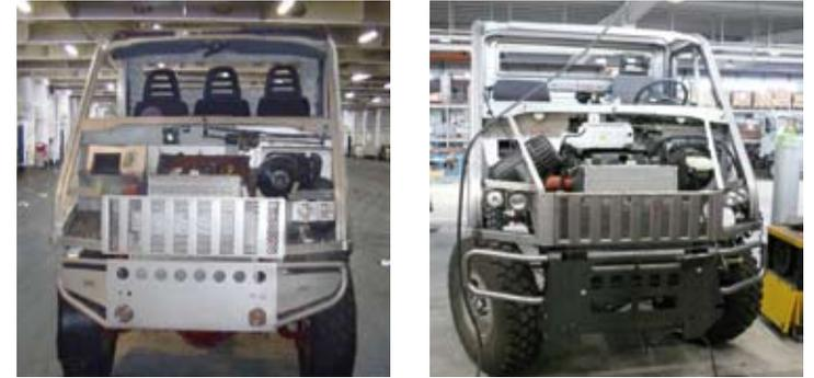
BREMACH developed series of models and prototypes to verify the virtual concept validity. The first prototype was in fact a static model for studies of the engine layout, ergonomics and habitability. After the first one, we made a series of working prototypes, on which had been tested several types of suspensions, engines, anchors.
