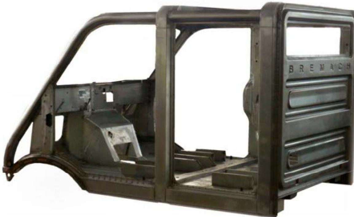
The new BREMACH vehicle is made with a cell of adaptive modular space frame. This frame is built up by tubular profiles which are worked in 3 dimensions in section to create a complex structure fitted out with a torsional resistance never achieved before on current vehicles.
