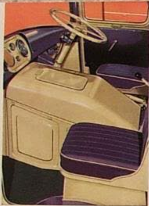
SEAT The driving seat is completely upholstered and manually adjustable fore and aft as well as for height.
