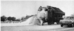
Ploughing and salt spreading automatically in the water tank of a motorway sweeper
