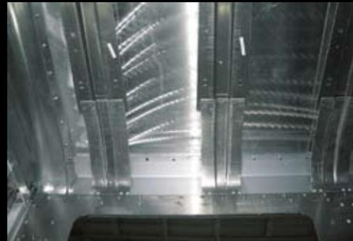
Roof constructed with .125" stamped roof bows on 15" centers for superior strength
