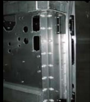
Aircraft-style Huckbolt construction maintains higher clamping force with extreme longevity
