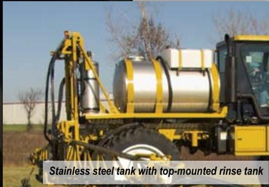
*Stainless steel tank with top-mounted rinse tank*
