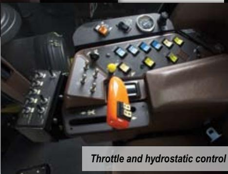
*Throttle and hydrostatic control*
